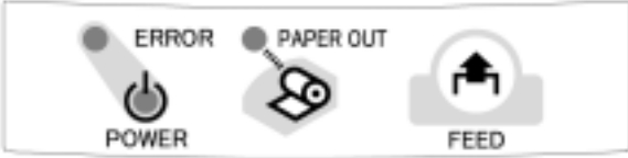
Figure 3.4.1 Panel Switches and Indicators
