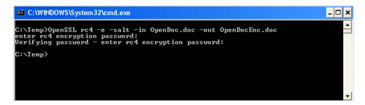
In the above example we have chosen to encrypt a Word document using the rc4 cipher with a salt. The size of the file is the document you are reading and is approximately 22MB. This encryption only takes a few seconds to complete. The next example shows the decryption of the same file.
