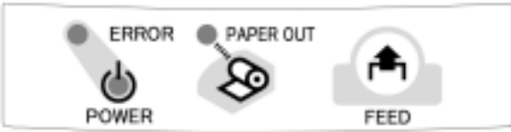
Figure 3.4.1 Panel Switches and Indicators
