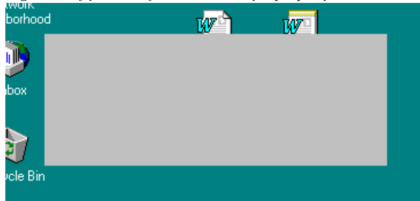
Figure A: If you set a form's BorderStyle property to bsNone , the form's borders will disappear.
