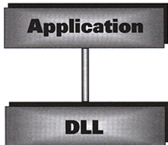
Figure A: Here's a typical application/DLL relationship.
